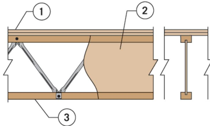
1. **Finished Flooring:** A double wood floor consisting of a subfloor of nominally 1-inch-thick (25.4 mm), tongue-and-groove wood-based, structural-use or 32/16 span-rated wood-based, structural-use (Exposure 1); and a second layer of nominally 1-inch-thick (25.4 mm), tongue-and-groove finish flooring. Alternatively, the finish flooring is permitted to be 40/20 span-rated wood-based, structural-use (Exposure 1), or Type I, Grade 1, particleboard not less than 5/8 inch (15.9 mm) thick.
