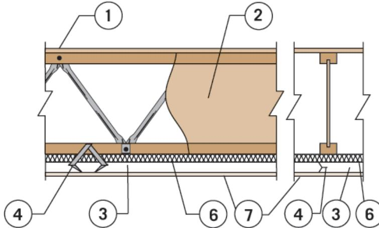
1. Finished Flooring: The flooring must consist of a single layer of 48/24 span-rated, tongue-and-groove, wood-based, structural-use (Exposure 1). When used as a roof-ceiling assembly, a single layer of square-edge, span-rated wood-based, structural-use (Exposure 1), complying with the code, is permitted to be used for roof sheathing. All butt joints of the sheathing must be located over framing members.
