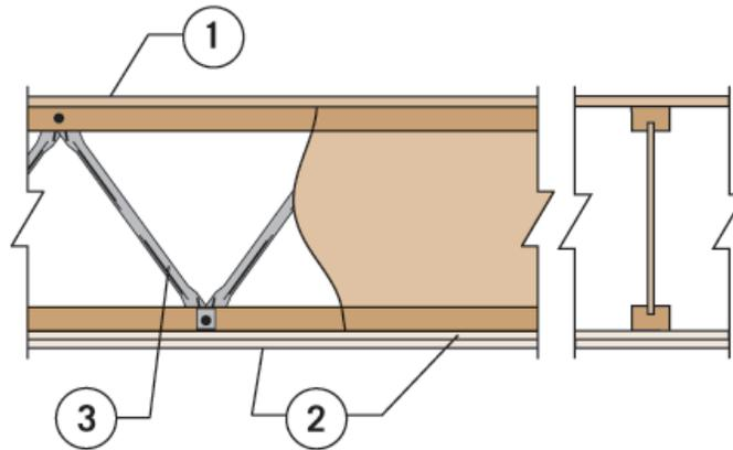
1. **Finished Flooring:** The flooring must consist of a single layer of 48/24 span-rated, tongue-and-groove, wood-based, structural-use (Exposure 1). When used as a roof-ceiling assembly, the decking is permitted to be any wood deck recognized in the code. All butt joints of the sheathing must be located over framing members.
