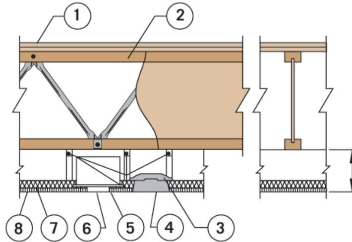
1. **Finished Flooring:** A double wood floor consisting of a subfloor of nominally 1-inch-thick (25.4 mm), tongue-and-groove wood-based, structural-use or 32/16 span-rated wood-based, structural-use (Exposure 1); and a second layer of nominally 1-inch-thick (25.4 mm), tongue-and-groove finish sawn lumber flooring. Alternatively, the finish flooring is permitted to be 40/20 span-rated wood-based, structural-use (Exposure 1). All butt joints of the sheathing must be located over framing members.
