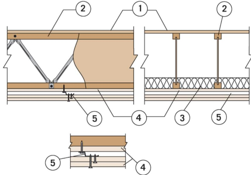
When use is as a floor-ceiling assembly over unusable crawl spaces, the ceiling membrane is permitted to be omitted. Additionally, flooring is permitted to be omitted where unusable attic space occurs above the system, provided the requirements of lateral support for compression edges are met.
