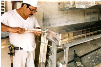
*Fleetwood worker builds a duct to the Energy Star® standard to assure air tightness in the air distribution system.*
