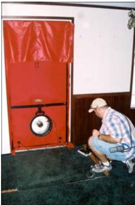
Tim Smiley, conducts a blower door test to measure whole home air leakage rate.
